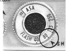
NOTE: If it is impossible to reach a desired ASA number or shutter speed setting, it is because of the interlocking of these two dials. A proper change in the setting of one dial will permit the other dial to be turned to the desired setting. For example, an ASA setting of 400 can only be made at shutter speed settings of 125 and 250.
